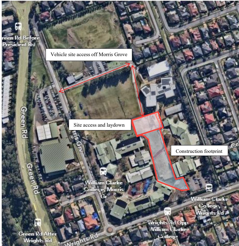
Figure 5-1 Site layout - Construction
