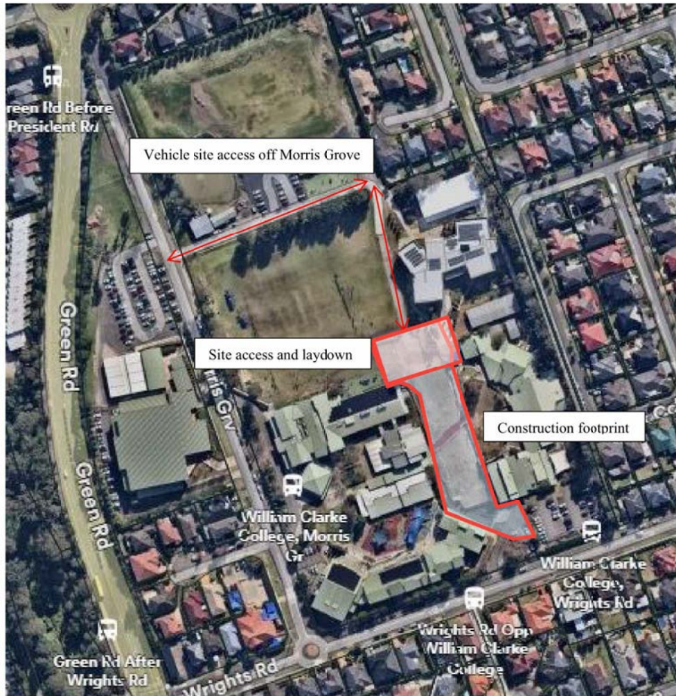
Figure 5-1 Site layout - Construction
