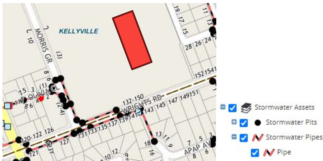
Figure 1-2 Council stormwater assets
